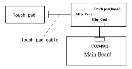
If the connection is loose, reconnect firmly. If there is still an error, go to Check 4.
